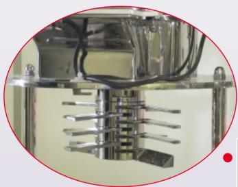
Multiple blade design to provide high performance milling. The PSM has a multiple blade design to give high performance milling and can be rapidly dismantled for product change and cleaning validation.
